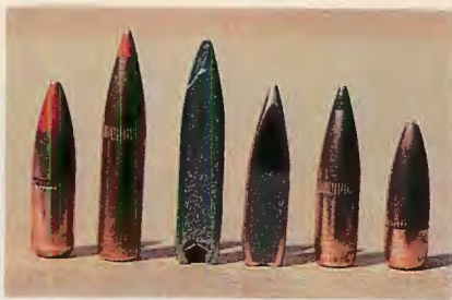
The old and the new: 1) Old M196 tracer projectile as used in M16A1 AR; 2) new L110 tracer projectile as used in M249 SAW; 3) L110 Tracer in cross section, showing large amount of trace element and gilded metal-clad steel jacket which allows 900-meter tracer burn; 4) SS109 ball projectile cross section (with hardened-steel penetrator and lead base) which allows penetration of U.S. steel helmet at 1,100 meters; 5) SS109 ball projectile with green-tip color code; 6) current issue M193 ball projectile.
